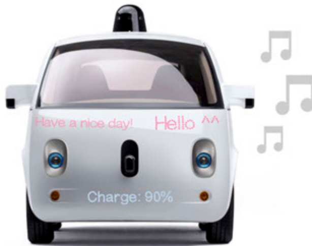
Figure 4.7: Bonnet and fenders fitted with LEDs and sound signalization
