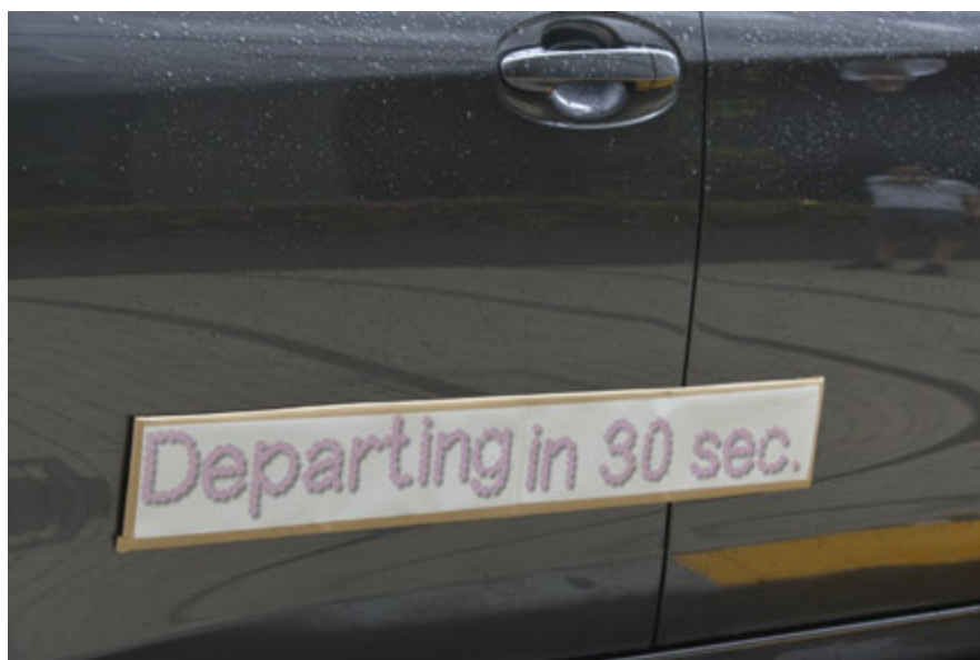
Figure 4.15: Distracted pedestrian alerted by the car with text, sound and icon on the side
