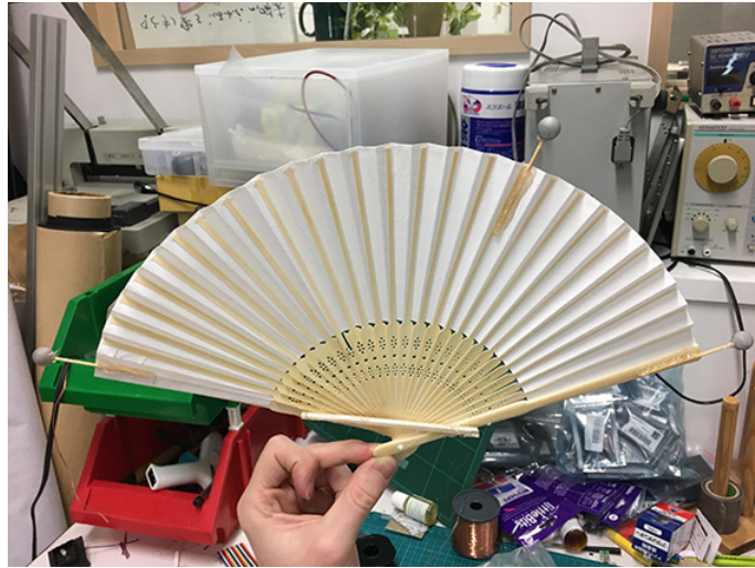
Figure 4.16: Folding Fan with Optitrack Motion Markers
