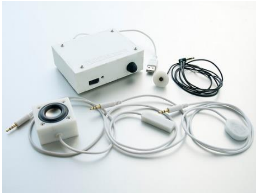
Figure 27: The TECHTILE Toolkit used to create gloves for one of the prototypes [57]
