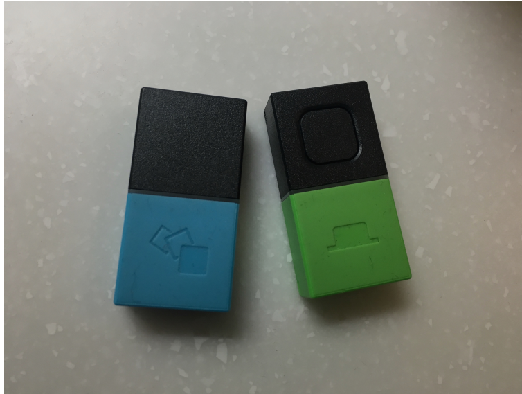
Figure 3.12: The Green “ Button ” Tag and Blue “ Move ” Tag from Sony Mesh Prototyping Tool
