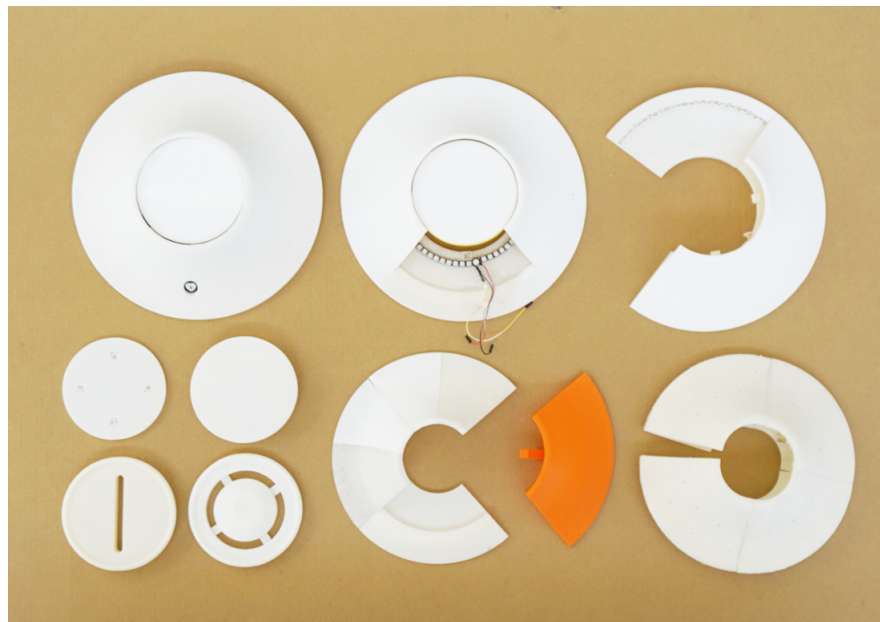
Figure 3.9: Hardware outer shell and internal mounting system prototypes and final (top left)
