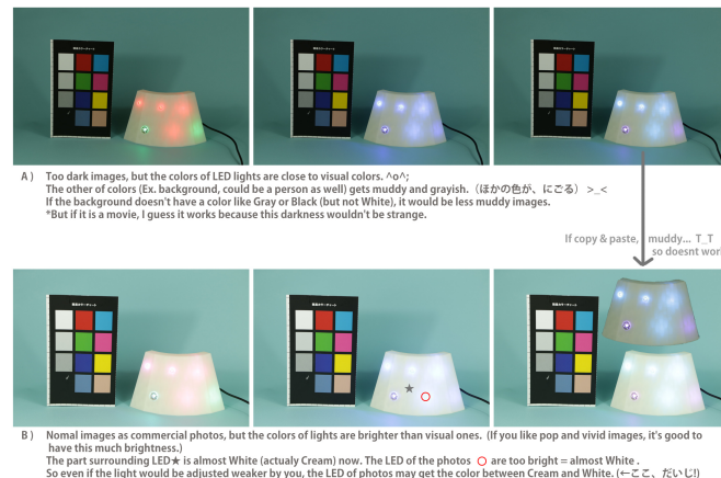
Figure 3.8: Early light testing with 3D print materials and patterns
