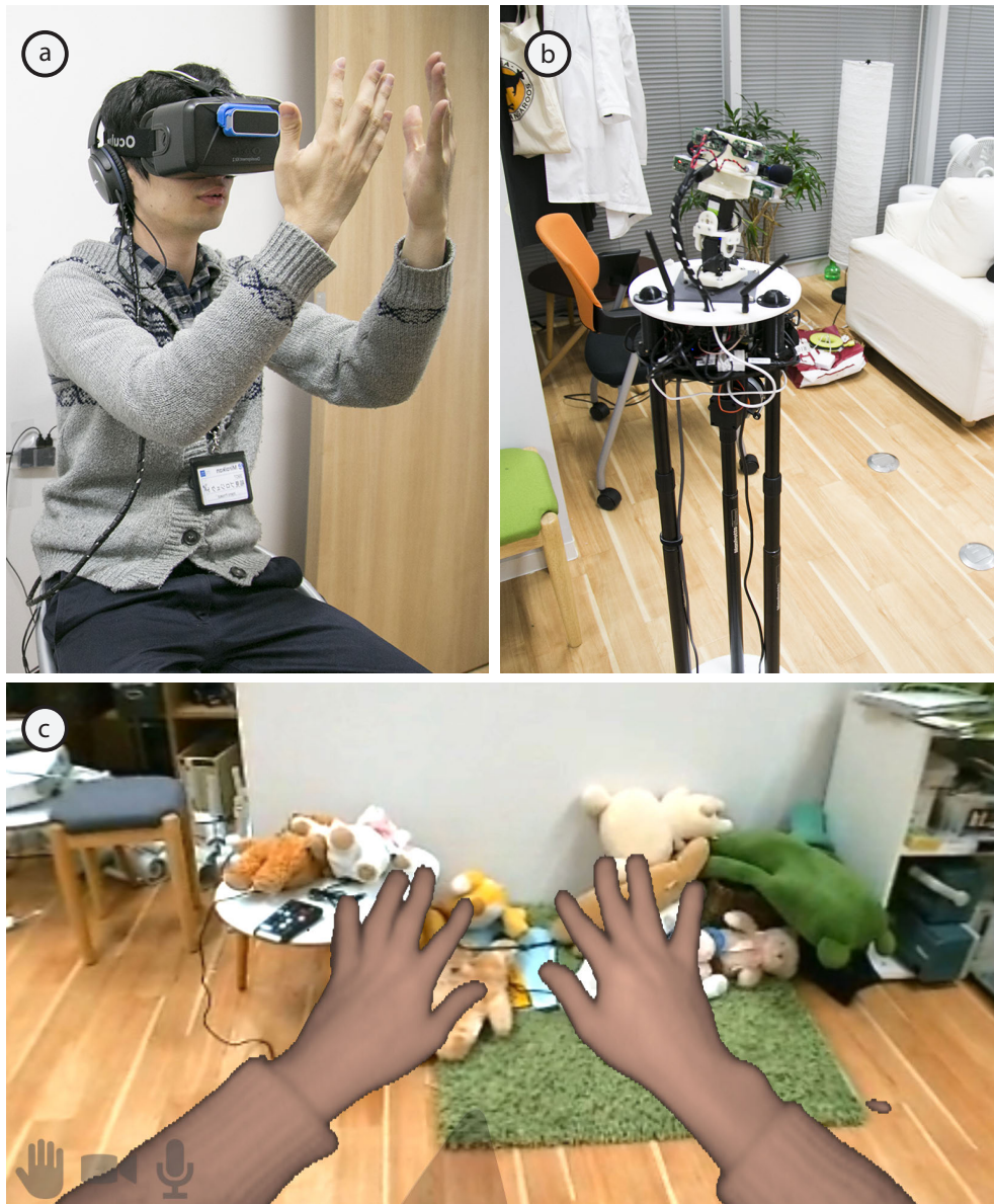
Figure 3.2: (a) A user looking through robot eyes in a different place, (b) Robot placed in a different environment, (c) First Person View of what the user sees.
