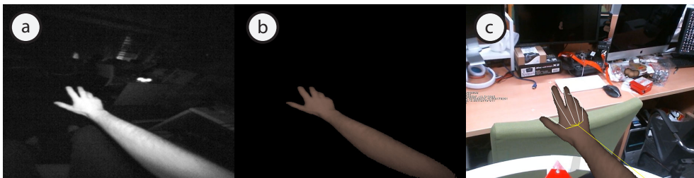
Figure 3.14: (a) Captured hands from Leapmotion (b) Processed image, remove background (c) Final superimposed hands
