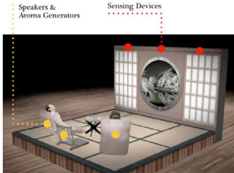
Figure 3.35: Sensing devices installed invisibly on top of the screen while aroma generators and speakers are embedded in the furniture
