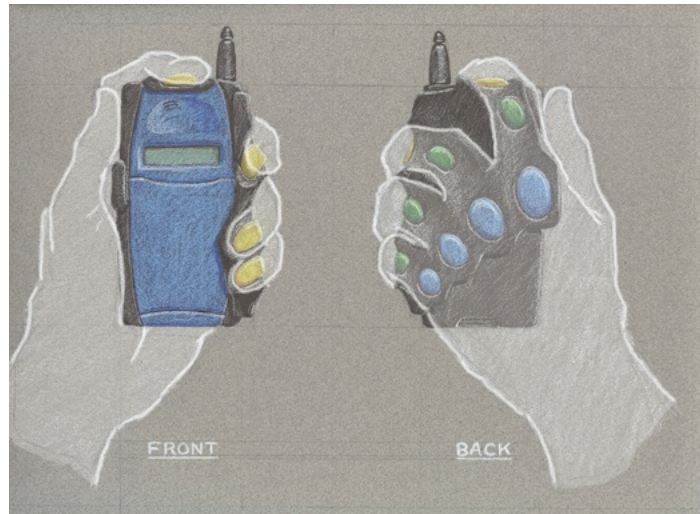
Figure 2.1: ComTouch Concept drawing showing a handheld sleeve that fits onto the back of a mobile phone
