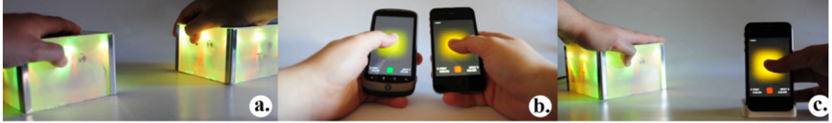
Figure 2.3: cubble 's hybrid interaction (holding hands). a. hardware only. b. mobile only. c. hardware and mobile combined.
