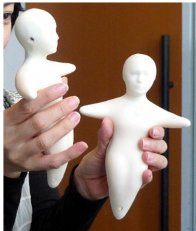
Figure 2.2: Portable human-like robotic avatar “ Elfoid ”, designed to convey individuals ’ presence
