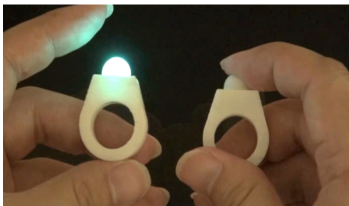
Figure 3.1: Squeezing the ring to send a lighting and a vibro-tactile signal to the paired partner.
