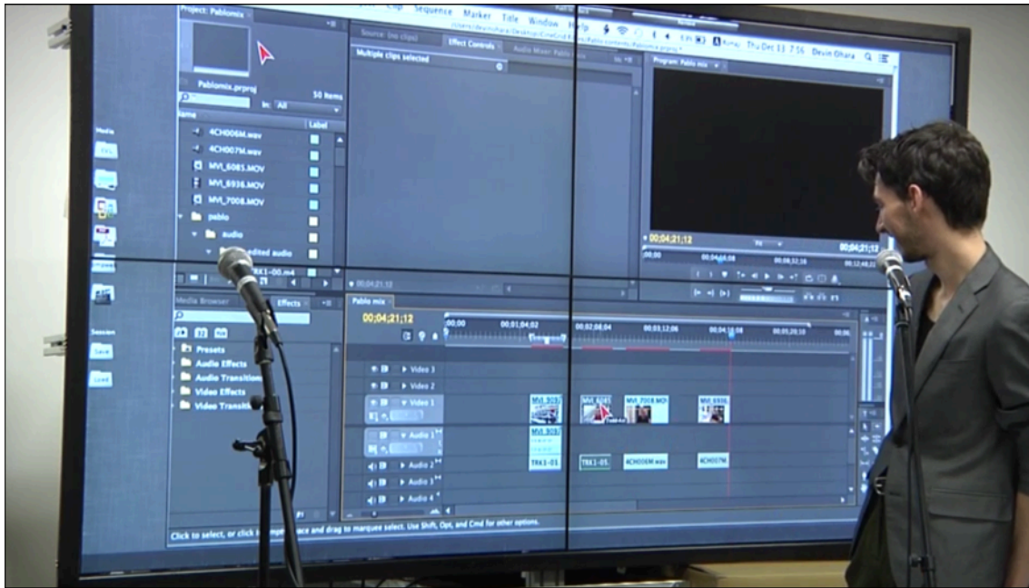
Figure 2.3. Shared applications from a PC/Mac can now be controlled on SAGE by different users using the SAGE pointer
