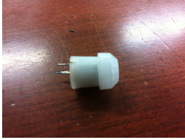
Figure 3.17: NaPiOn sensor , slight motion detection type
