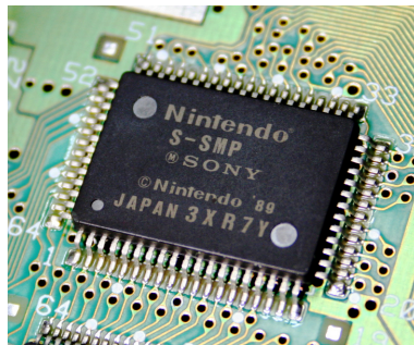
Figure 2.3: S-SMP Sound Chip
