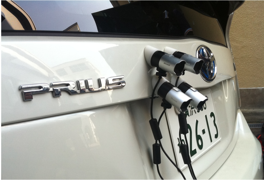
Figure 3.11: Four cameras fixed at the rear of the car.
