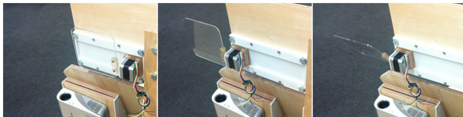
Figure 5.5: Half mirror display integrated to headrest; (a)hidden position, (b) extended position and (c) mirror rotated to an appropriate angle.
