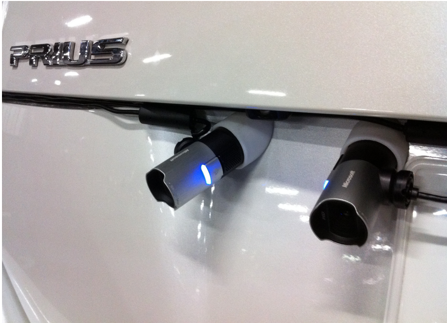
Figure 3.6: Two cameras fixed at the rear of the car.
