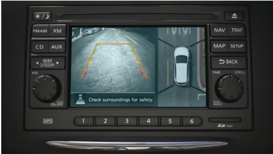
Figure 2.9: Nissan Around View Monitor.
