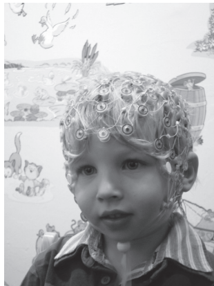
Figure 1. Young child wearing a high-density (128-channel) electroencephalography (EEG) Sensor Net (Electrical Geodesics, Inc., Eugene, Oregon) for a study of face versus object processing. University of Birmingham, England. Photo Credit: Antonis Christou.
