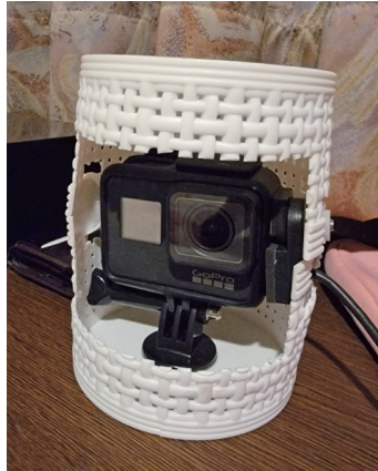
Figure 17: The first makeshift container created by Corey Noxon to shade the timelapse camera to prevent overheating. (19 August 2024)
