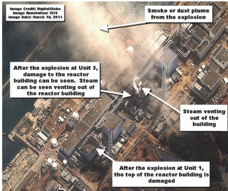
Figure 1.3 Observation of Fukushima Daiichi Nuclear Power Plant by Worldview-2 satellite of DigitalGlobe, Inc.(Photographed on March 14, 2011)<sup>[3]</sup>
