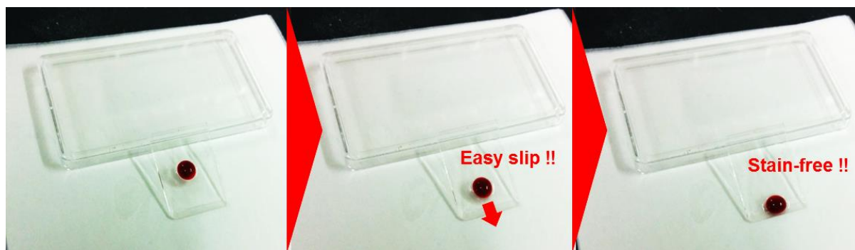
Figure 4-19. Pictures showing how blood was repelled from the biocompatible SLIPS after it was dropped (left), as it was sliding (centre) and after it slid off (right). Reproduced with permission from Ref [132]. Copyright 2015 American Chemical Society. 132
