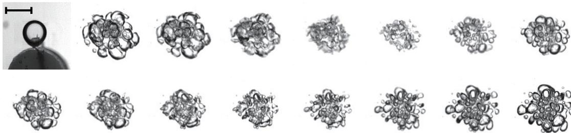
FIGURE 3.5: A typical image sequence of an oscillating bubble cluster driven at 625 Hz. The image sequence corresponds to one oscillation cycle of the imposed driving frequency. The scale bar represents 2 mm.
