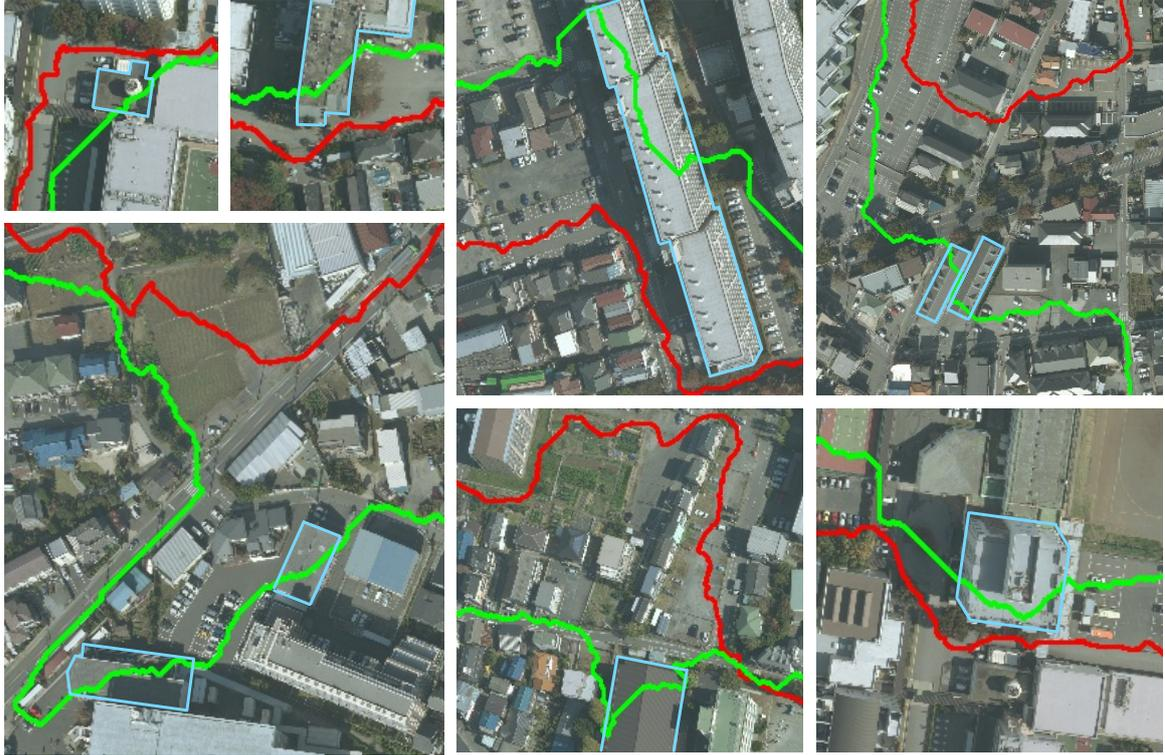
Figure 6-6: Red lines show the seamlines found by our method. Green lines show the seamlines found by the conventional method[Pan et al., 2014]. The light blue lines denote buildings that are passed through by seamlines.
