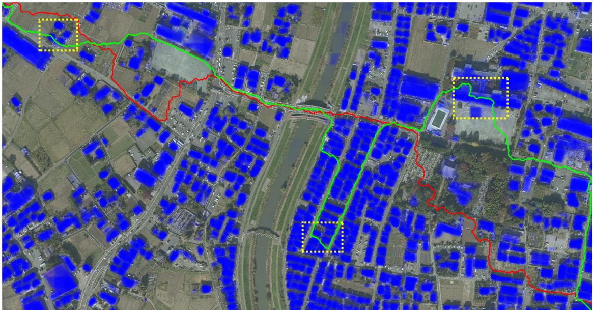
(b) This is another example result. Red and green lines and yellow rectangles have the same meaning as in Figure 6-7a. In the right-most yellow rectangle, the green line drawn by the conventional method passes through a large building even though the ground beside the building is larger.
