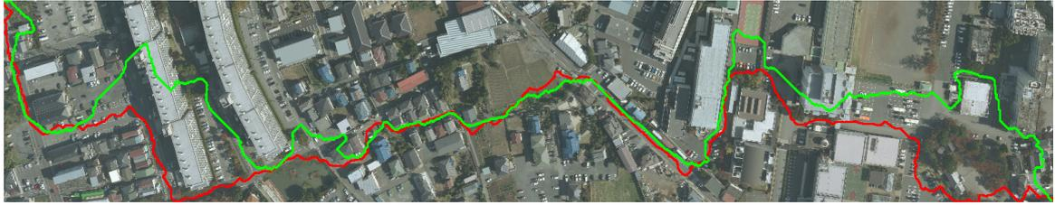
(a) The green line and the red line show the seamline found by the conventional method [Pan et al., 2014] and the seamline found by our method, respectively. Both seamlines are drawn on an input aerial image.
