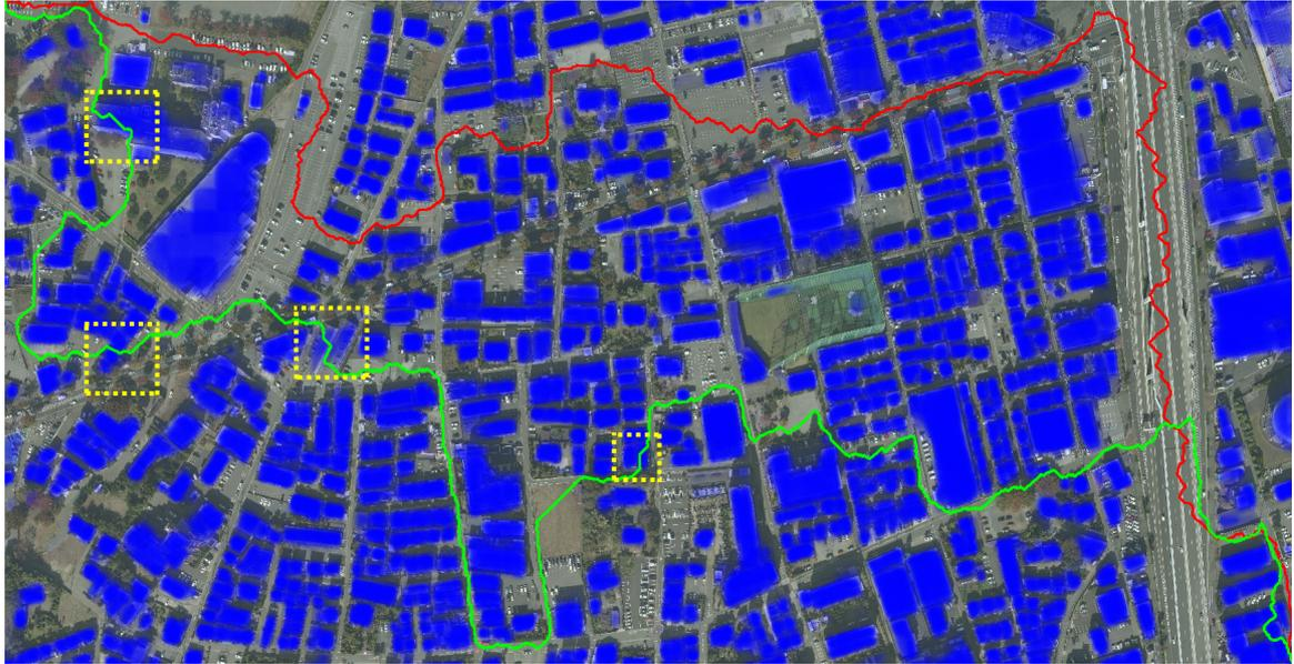
(a) Red lines denote the seamlines determined by our method. Green lines denote the seamlines determined by the conventional method [Pan et al., 2014]. The red lines pass through many parking areas and roads, while the green lines pass through residential areas. Yellow rectangles indicate the existence of buildings passed through by the green seamlines (the conventional method).
