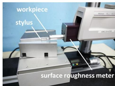
**Fig. 7-10 Surface roughness meter.**
