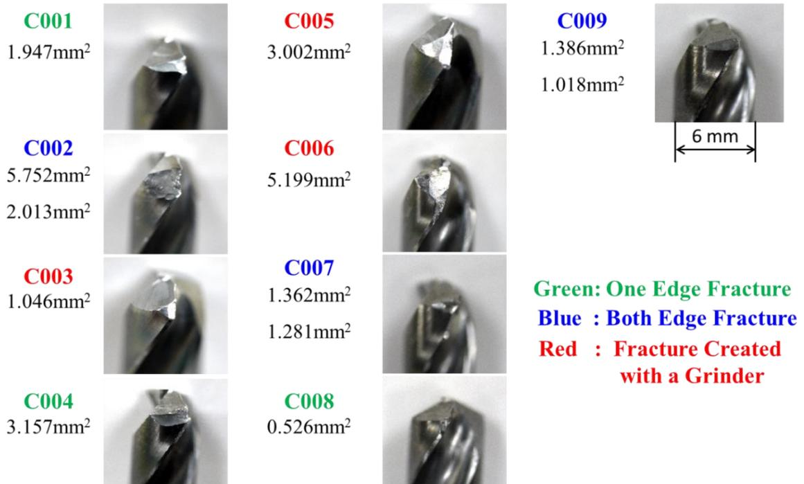
**Fig. 6-9 Appearances of fractured drills.**
