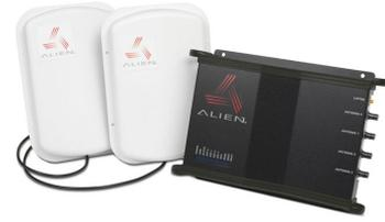
(c) UHF RFID reader (cited from [www.barcodesinc.com](http://www.barcodesinc.com))
