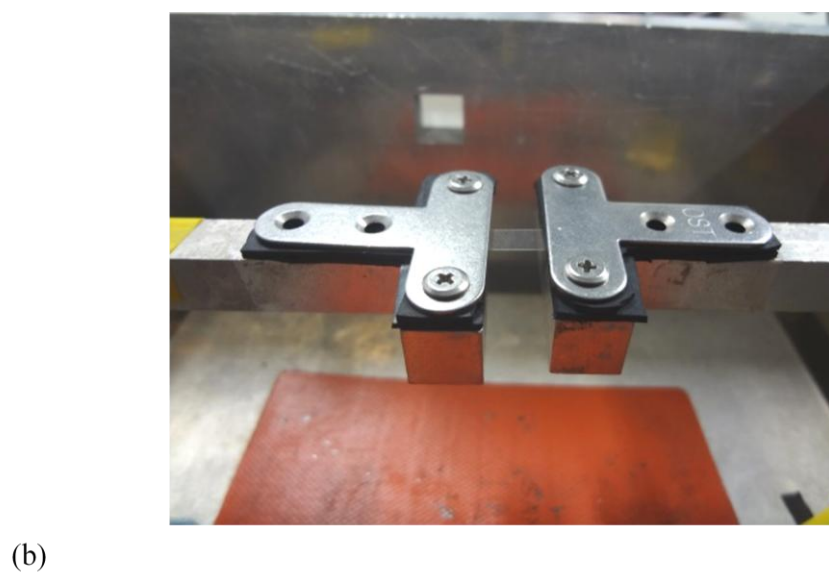
Fig 3.1 Experimental setup for characterization of Nafion: (a) Overview; (b) Close-up of the gripping mechanism
