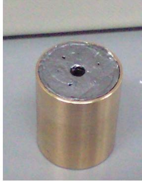
**Fig. 3.12:** The sample after being glued into the cap.
